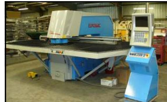
*CNC Turret punch for punching of sheet material*
