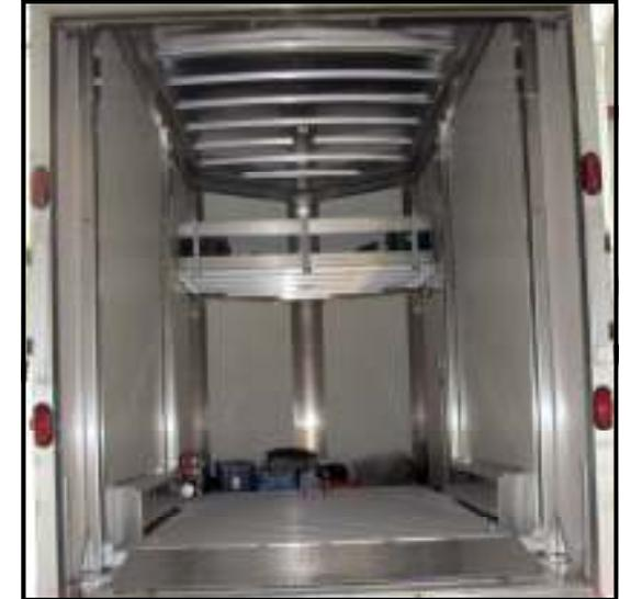
*Lift in lowered position showing front upper deck*
