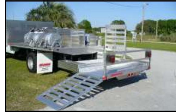
*Spray truck dual rear spreader platform with side load ramps and bucket rack*
