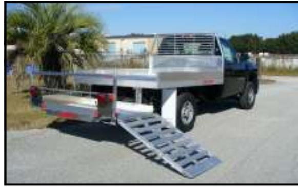
*Model 1222XL312K Flatbed with rear spreader platform with side load ramps and bucket rack*
