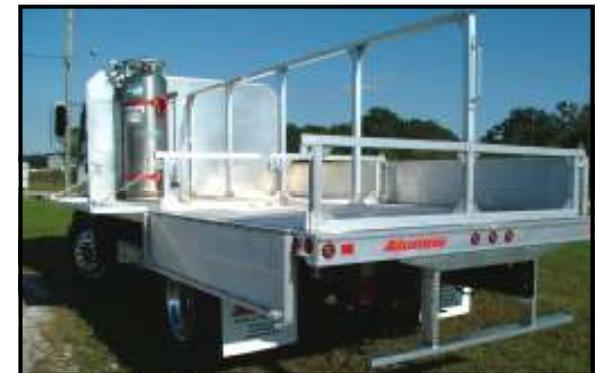
*Fish Tank body with fold down sides & air line rack*
