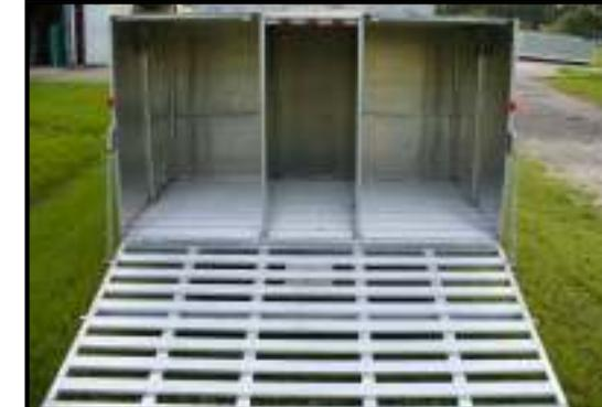
*Spray truck rear enclosed spreader boxes with center storage*
