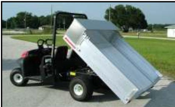
*Tilt for dumping and engine access*
